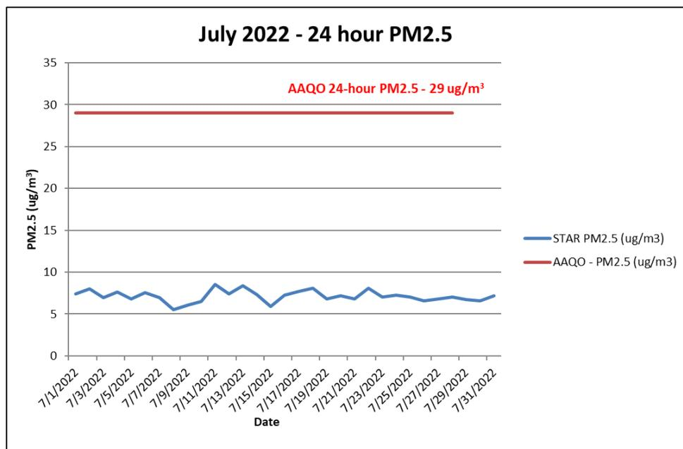
Figure 4: 24-hour concentrations of PM<sub>2.5</sub> at STAR
