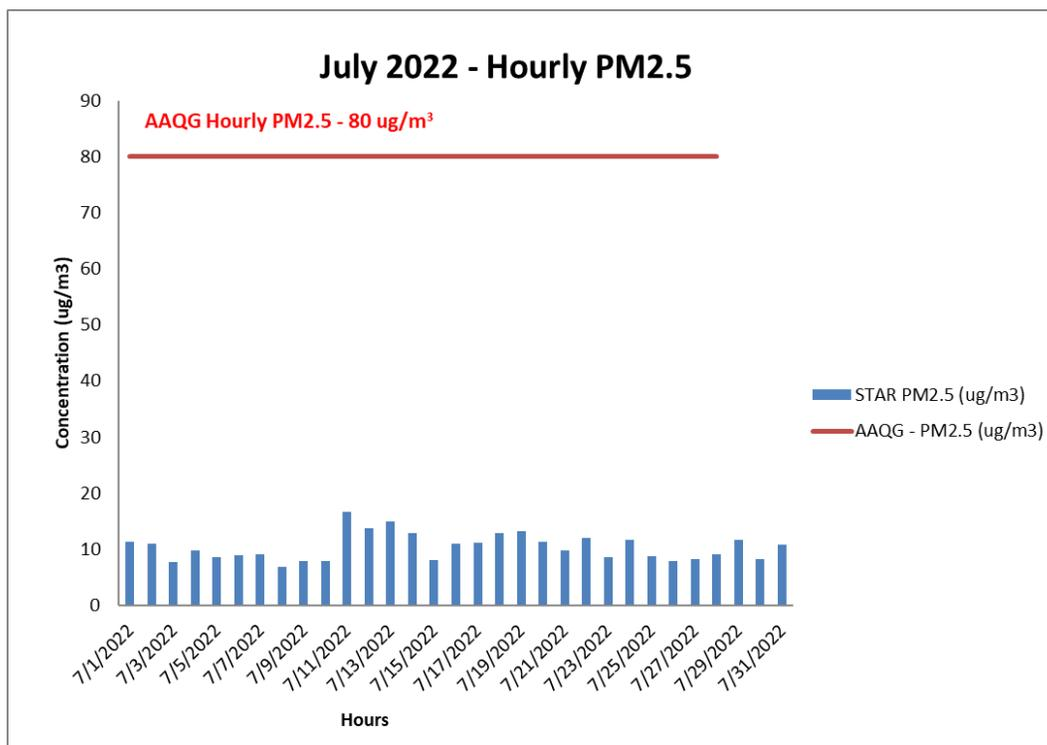
**Figure 2: 1-hour concentrations of PM<sub>2.5</sub> STAR**
